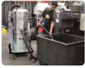
Compressed air vacuums are the ideal solution in ATEX zoned areas, for maintenance, general cleaning, and for collection of organic and metallic dusts, and swarf containing explosive vapours.
